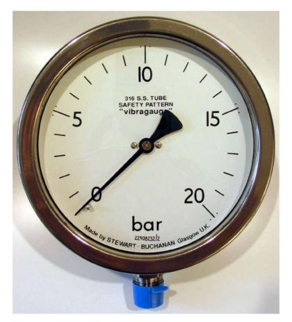
This gauge has been specially developed to meet the problem of excessive vibration which is the biggest single contributory factor in limiting the life of the instrument. It also helps to protect against the problems associated with rapid surge or loss in pressure and trying to obtain an accurate reading from a fluttering pointer due to pulsation.
